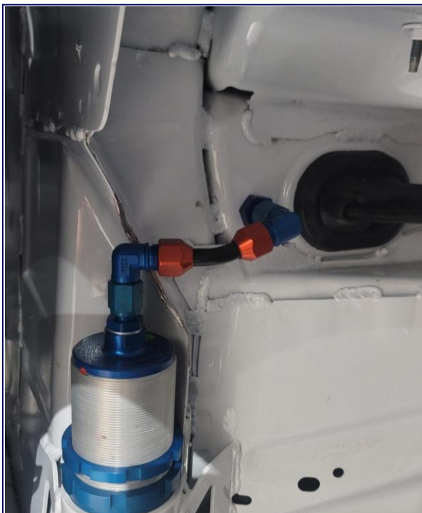
Front Air Jack / Bulkhead Connection Passenger Side
