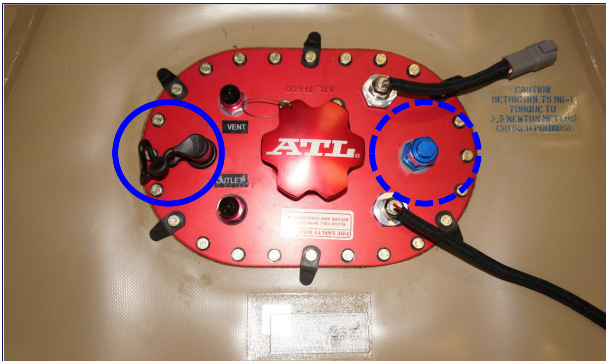
Fuel Cell Fitting Location
