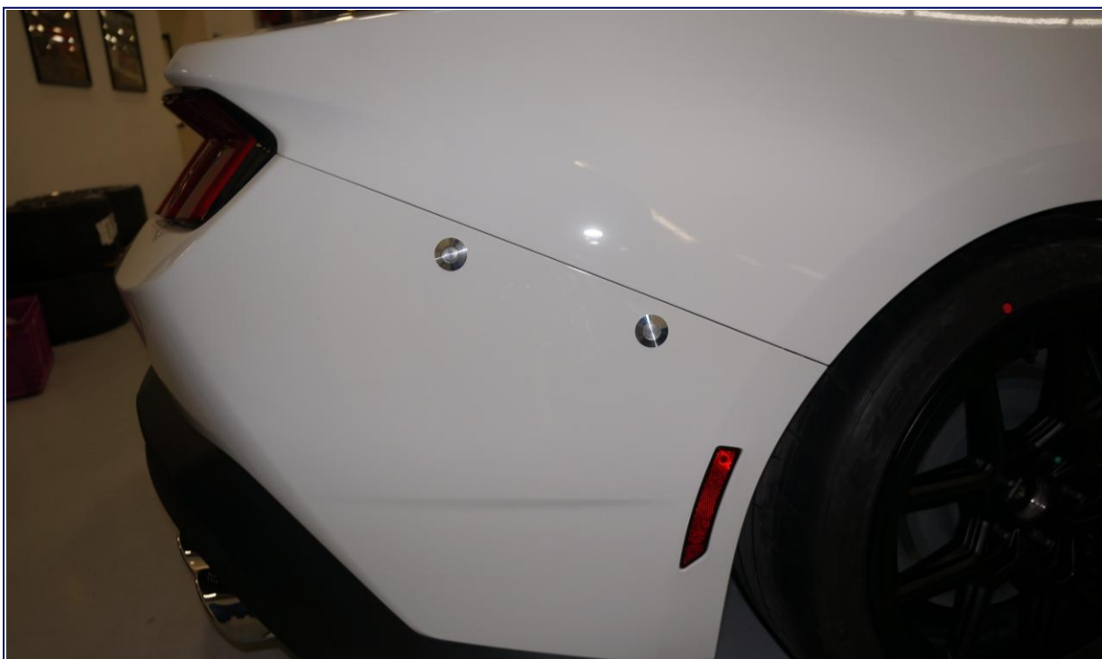
Rear Fascia Mount Repair Only repair allowed for damaged rear fascia corner mounts
