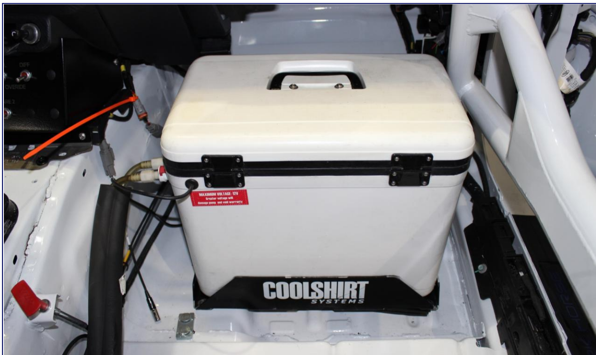
Driver Cooling System Location Passenger Side Footwell
