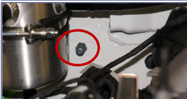
Engine Bay Nozzle 2 Passenger Side
