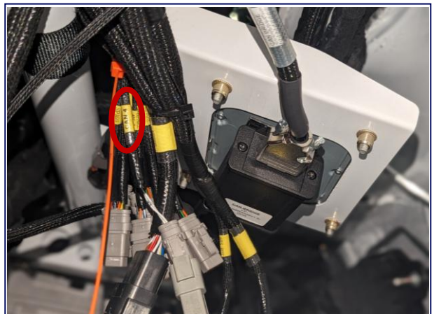
VBOX Wiring Labeled "CAN4" Underneath Dash
