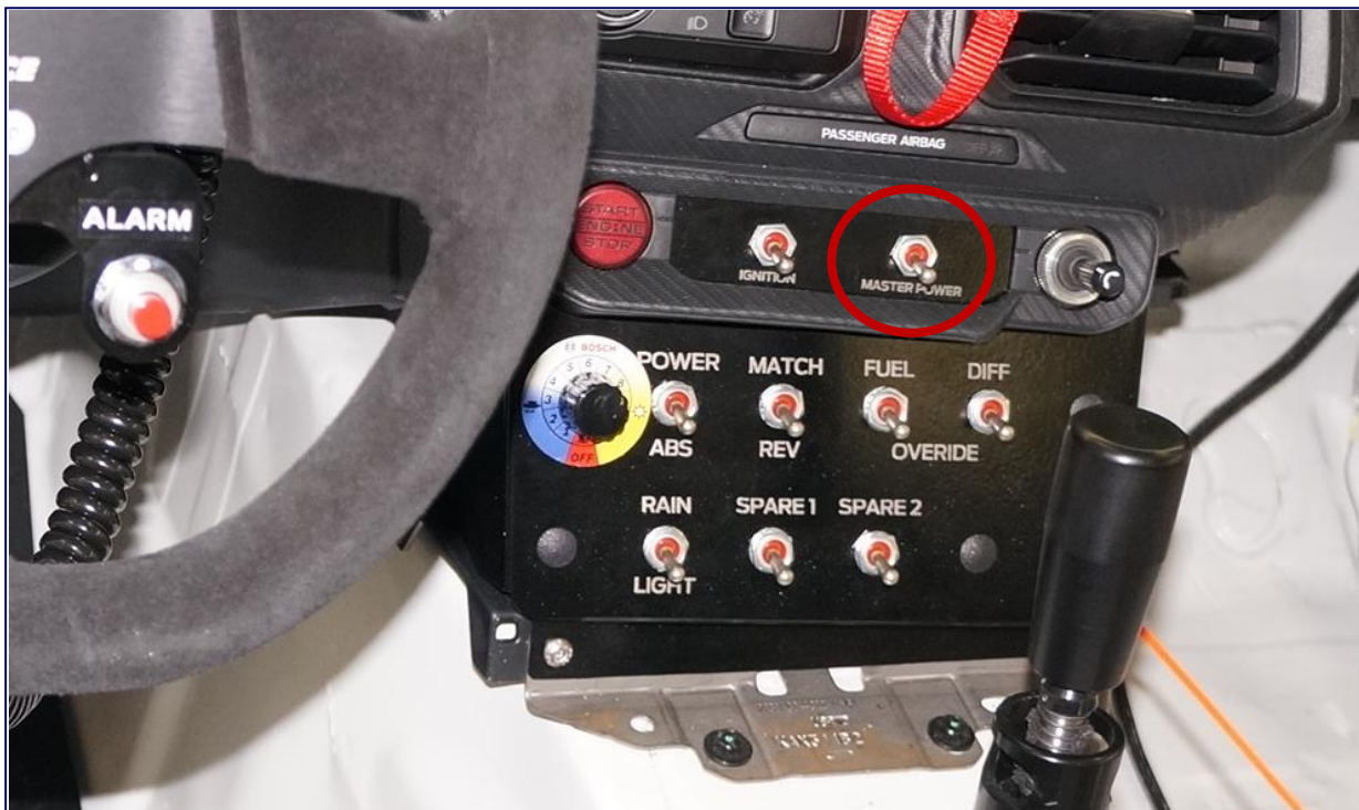
Interior Master Power Electrical Switch OFF – Down towards Floor / ON – Up towards Roof
