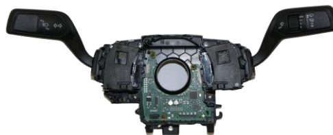
Multifunction Switch DHR-CLMNSWCH-MOD
