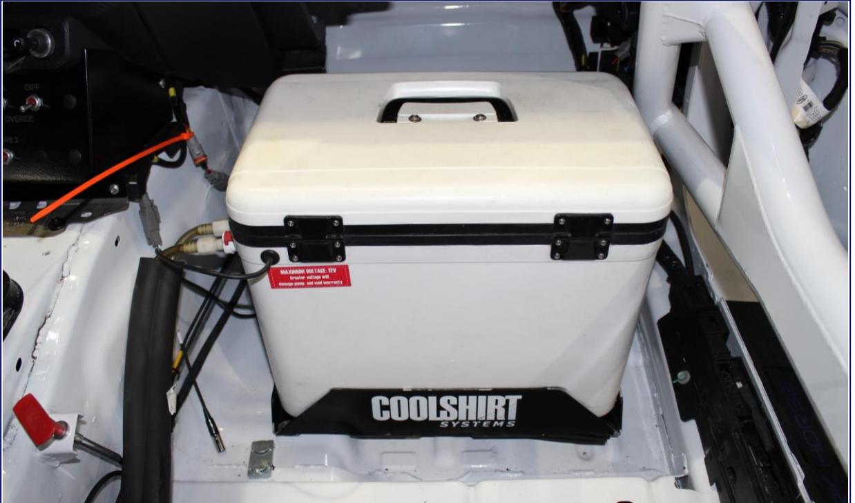
Driver Cooling System Location Passenger Side Footwell
