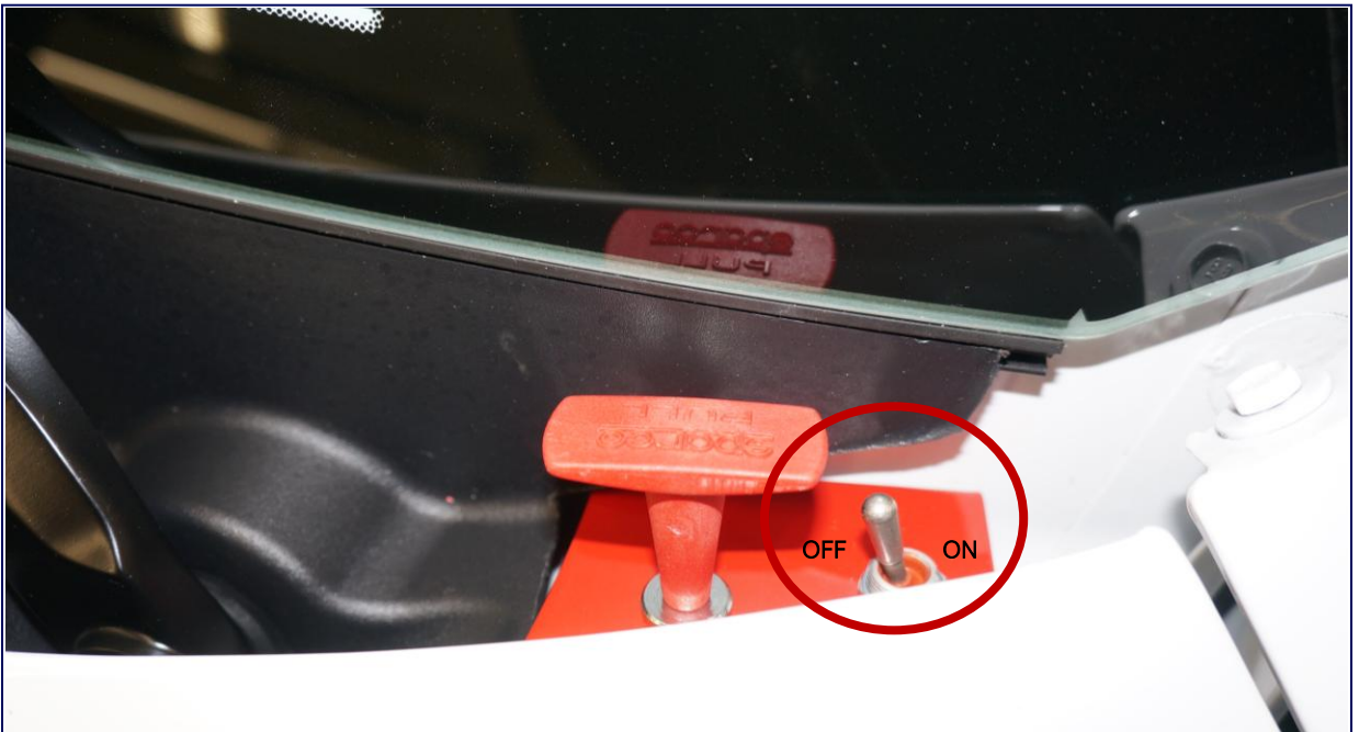
Exterior Master Power Electrical Switch Exterior Driver Side OFF – towards Passenger Side / ON – towards Driver Side
