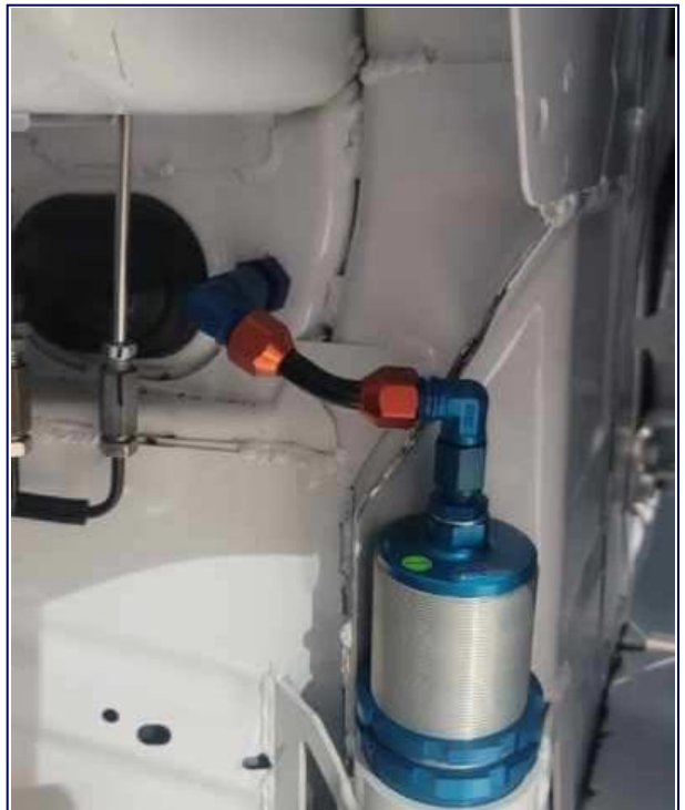
Front Air Jack / Bulkhead Connection Driver Side
