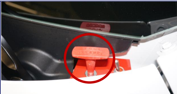
Exterior Cable Pull Exterior Driver Side
