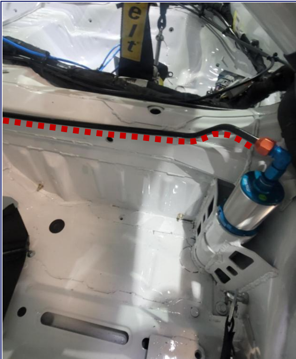
Rear Air Jack Driver Side
