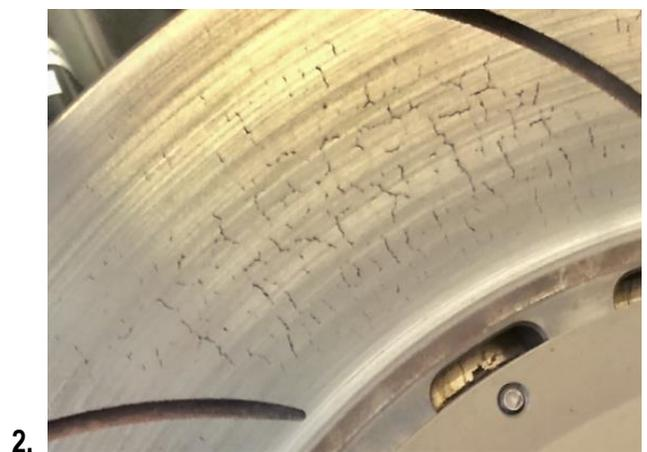
A rotor that has been used and / or run at a higher temperature range will exhibit “stress cracks” on the rotor outboard and inboard surfaces only (picture 2, above right). Continued use will cause these “cracks” to grow in length, which is considered normal. If the cracks propagate around the OD or the ID of the rotor then it is considered no longer usable and must be changed.
